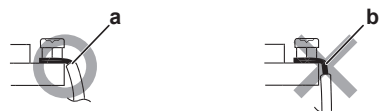
a Strip wire end to this point b Excessive strip length may cause electrical shock or leakage.
